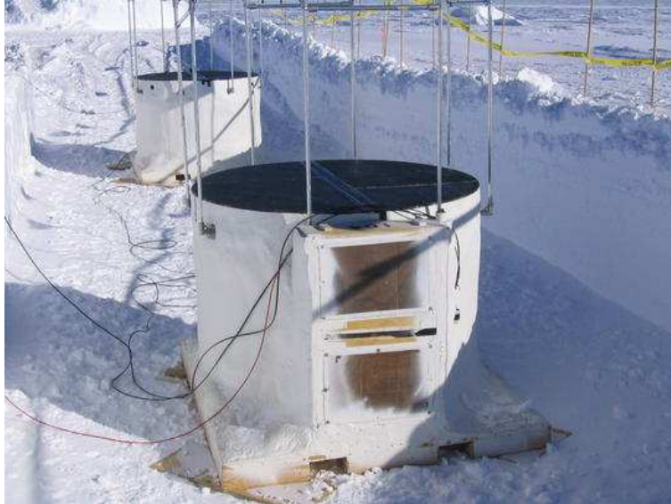
Figure III.5: The IceTop detector tanks
